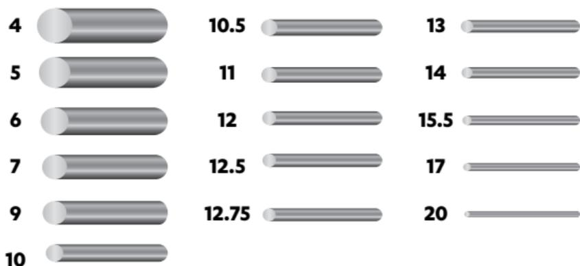
THE LOWER THE NUMBER ASSIGNED TO A WIRE THE LARGER ITS DIAMETER.
